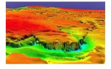
the land submerged by Celilo Lake, and the results were a pleasant surprise. Clearly visible on the sonar are the basalt cliffs over which Celilo Falls fell. Resting virtually intact under the lake's surface. Although it may be unlikely that the Dalles Dam will ever be removed and the falls restored, the very fact that they endure gives some hope that the way of life they represented will not be forgotten.
