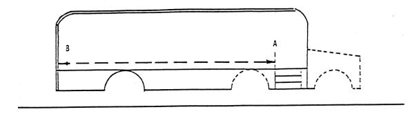
Forward engine transit or conventional with rear luggage compartment and standard rear seat. Measure from rear of stepwell to inside face of luggage compartment at floor level.
